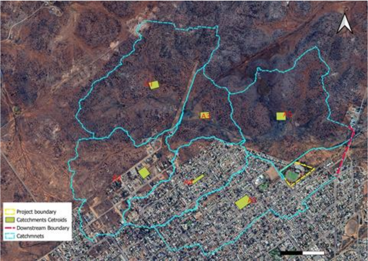
Figure 8- TUFLOW Model Setup
